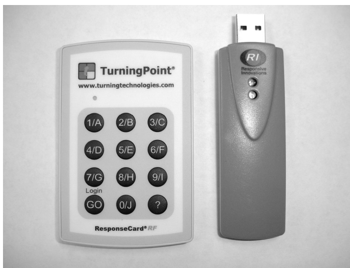
Figure 1 Audience response hardware from TurningTechnologies: student transmitter (left) and instructor receiver (right)
